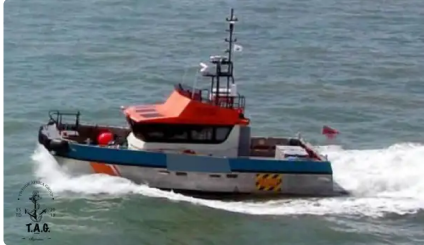
15m Waterjet Crew Transfer Vessel
