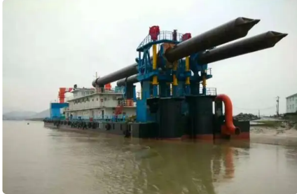
106.65m Cutter Suction Dredger 4500 cbm
